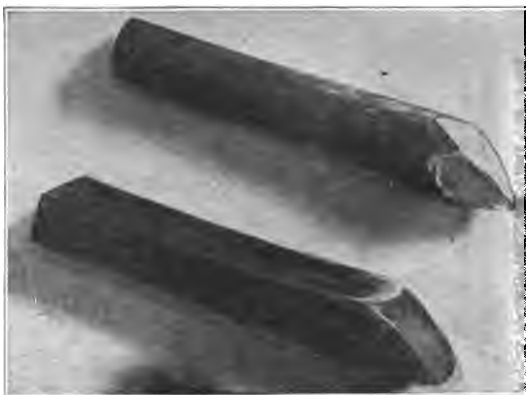
Fig. 27. Work Scarfed for Lap Weld
